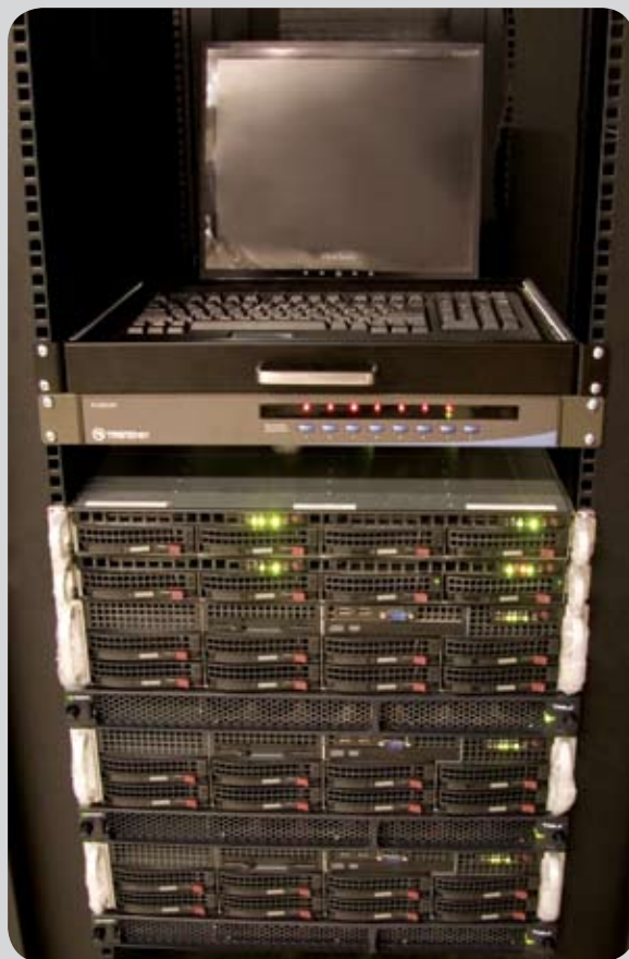
The standard Volera hardware configuration consists of 3 NVIDIA S1070s and is capable of processing the full OPRA feed in less than 10 milliseconds.
